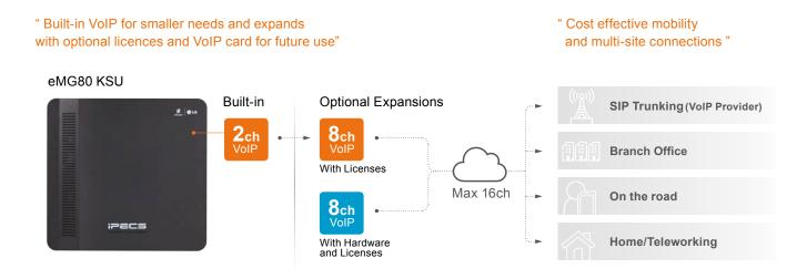
iPECS eMG80 is a hybrid TDM/IP system ideal for cost effective solutions. With its modular and flexible design, businesses can easily and affordably expand into Unified Communications and more sophisticated enterprise applications.
